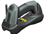
4. <u>Firmly position the handheld unit onto the cradle within 15 seconds.</u> A long beep and a short beep will be emitted to indicate a successful setting; otherwise, three short beeps will be emitted to indicate an unsuccessful setting.
