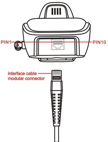
Figure 2-1 Cable connector interface pin-outs
