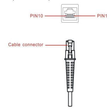
Figure 2-1 Cable connector interface pin-outs
