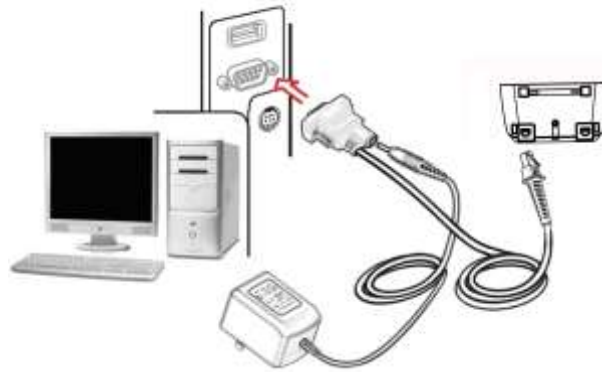
Figure 2-11 Installation of RS232 cable
